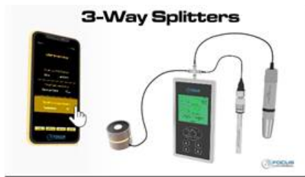
Figure 7, A pH sensor, a CO2 sensor and a light sensor are connected to the universal device and change it to a 3-sensor device. A computer or smartphone can also be used for display.
