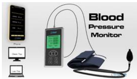
Figure 5. A blood pressure sensor is connected to our Universal Device we call the Ubiquitor and changes our device into a blood pressure measurement instrument.
