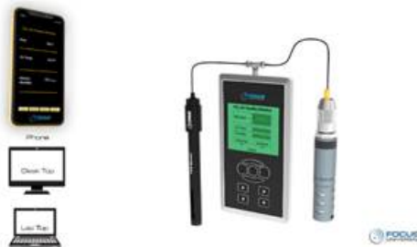
Figure 6. A pH sensor and a CO 2 sensor are connected to our universal device and our device changes into a split-sensor device. A computer or smartphone can also be used for display.
