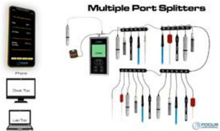
Figure 8, any number of sensors in any combination are connected to the universal device and change it to a multiple sensor device. A computer or smartphone can also be used for the display.
