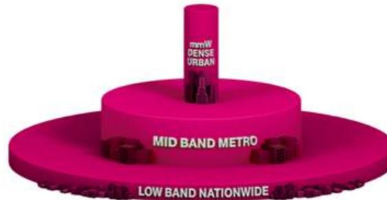
High-band, mmWave spectrum is used primarily for urban and dense urban markets. The characteristics of high-band, mmWave spectrum is that it is very wide and provides a significant increase in capacity. Because of the greater spectrum width, speed is increased, and transmission latency is reduced. However, the drawback is that high-band spectrum does not propagate over a large coverage area. For example, a 28 GHz mmWave spectrum can only travel 500 feet.<sup>10</sup>
