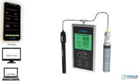
Figure 6. A pH sensor and a CO2 sensor are connected to our universal device, and our device changes into a two-sensor device. A computer or smartphone can also be used for display.
