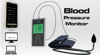
Figure 5. A blood pressure sensor is connected to our universal device, which we call the Ubiquitor, and changes our device into a blood pressure measurement instrument.
