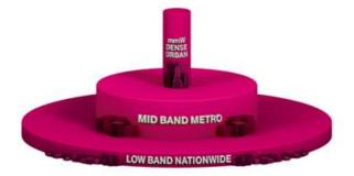
High-band, mmWave spectrum is used primarily for urban and dense urban markets. The characteristics of high-band, mmWave spectrum is that it is very wide and provides a significant increase in capacity. Because of the greater spectrum width, speed is increased, and transmission latency is reduced. However, the drawback is that high-band spectrum does not propagate over a large coverage area. For example, a 28 GHz mmWave spectrum can only travel 500 feet.<sup>10</sup>
