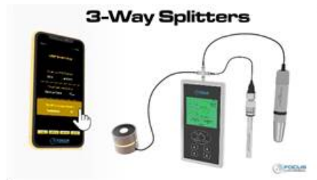
Figure 7. A pH sensor, a CO2 sensor, and a light sensor are connected to the universal device, and the device changes into a three-sensor device. A computer or smartphone can also be used for display.
